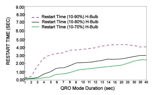
Figure 17. Restart Time Versus QRO State Duration, H-bulb
